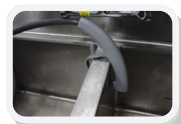
Hose and temperature sensor secured to suction cup.
