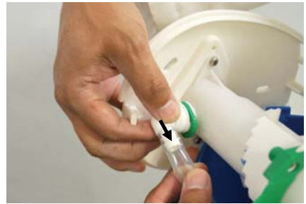
3.) For bottle versions only: discharge tube will need to be disconnected to remove cover
