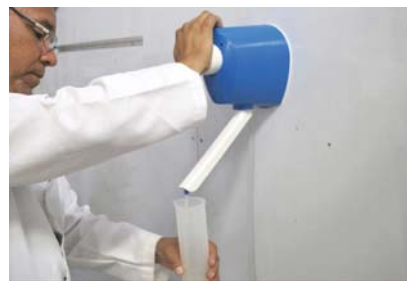
2.) Turn dial to 50 ml position and push dial. Repeat pushing action until DosaMAX Jr. is primed.
