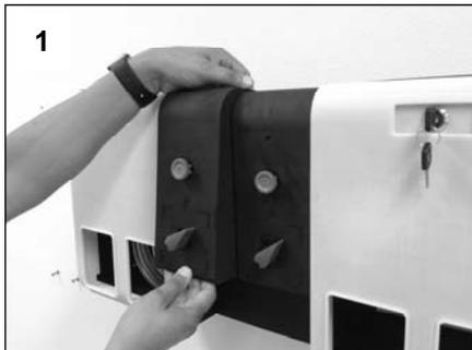
1 Snap off cover by gently pulling at the bottom and top of the cover. Repeat for the second cover.
