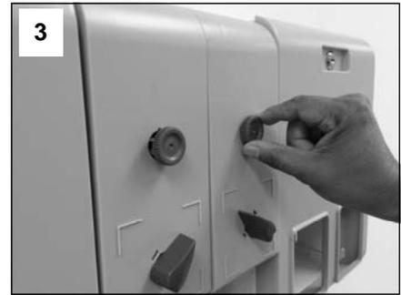
3 If desired, the button can be “locked” in the ON position for filling large containers such as mop buckets or floor scrubbers. Simply turn the button slightly clockwise when pressed in. To release, turn button counter-clockwise.
