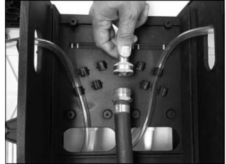
Attach male connector on high pressure supply hose to the proportioner. Water inlet can be located on the backside of the unit.
