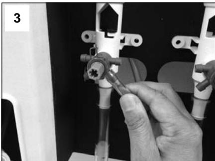
3 Take the 3/8" O.D. chemical suction tube and slide it over chemical inlet port. When ready, secure the tube onto the inlet port with the supplied zip ties.
