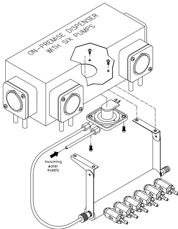
NOTE: The example shown above is for mounting the manifold to pump cases built prior to June, 2002.
