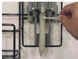
3. Install the appropriate metering tip(s) to the venturi body. Connect 3/8" O.D. vinyl chemical suction tube to the venturi, completely covering the metering tip(s).
