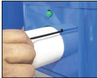
Dosing amount can be locked in place using a 3 mm hex driver
