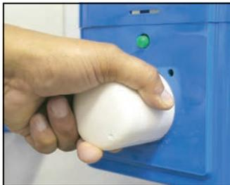
Turn the knob to select dosing amount ranging from 5 ml to 50 ml in 5 ml increments.
